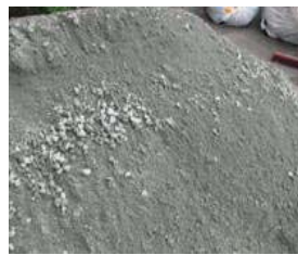
\frac{3}{4} " to \frac{1}{4} " Primary Base Drain Rock
