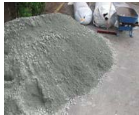
\frac{3}{4} " to \frac{1}{4} " Primary Base Drain Rock
